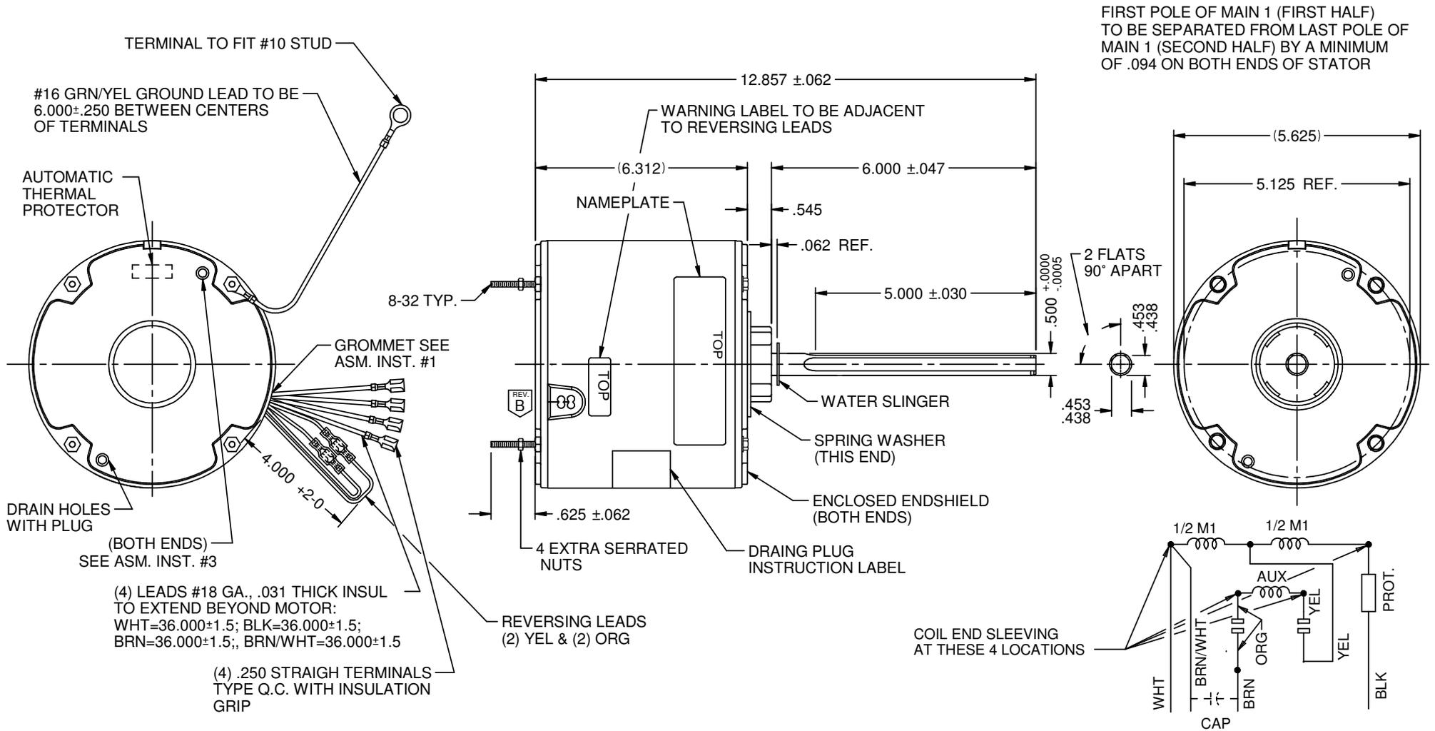
FIRST POLE OF MAIN 1 (FIRST HALF) TO BE SEPARATED FROM LAST POLE OF MAIN 1 (SECOND HALF) BY A MINIMUM OF .094 ON BOTH ENDS OF STATOR
